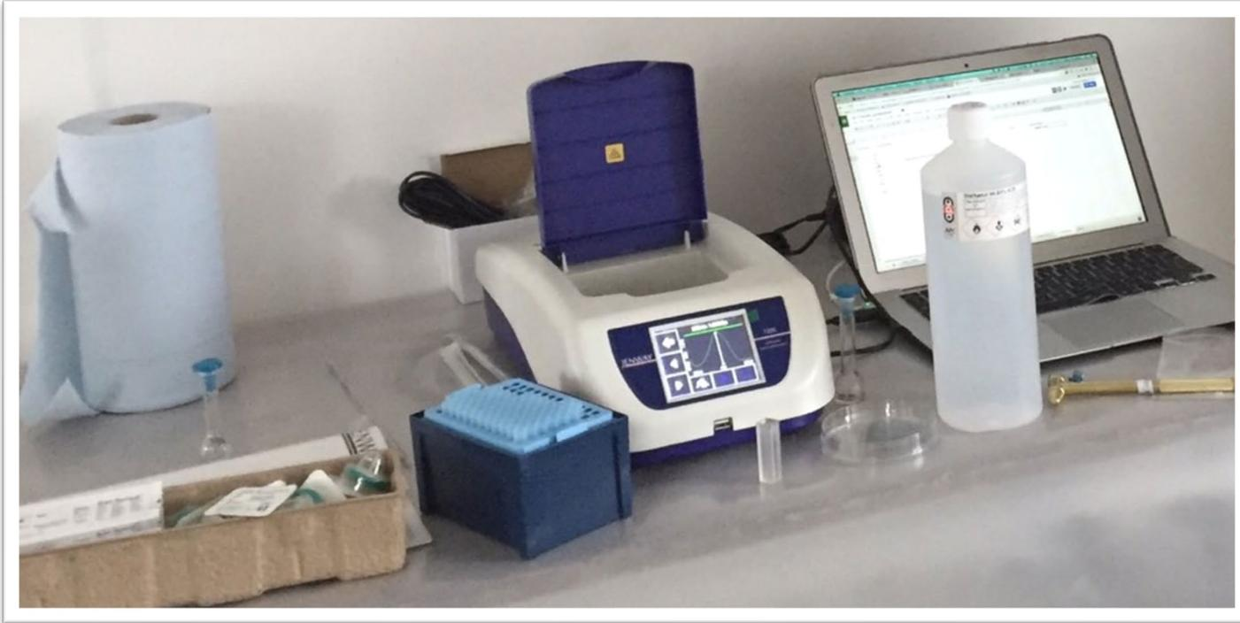
UV-Vis Spectrophotometry quantifies a solution of MDMA based on its absorption of ultra violet light
